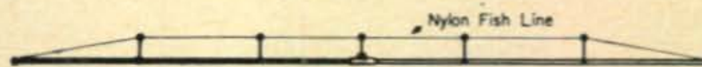
Fig. 2—The director and reflector would sag without the support shown above. Nylon fish line, 100 lb. weight, is stretched through five 5" TV stand-off insulators.
